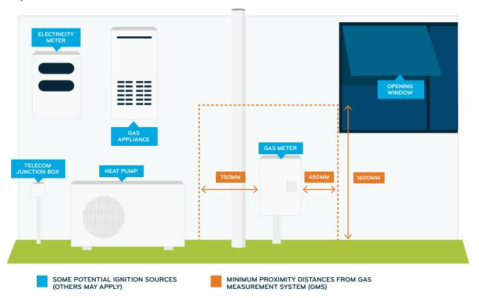
Please note that your gas connection should be unobstructed and easily accessible to us. No structures such as decks should block access to the gas connection. We cannot cut into a decking structure to access the gas connection as this may render the deck unsafe. However, this excludes concrete work around the connection as we are able to drill the concrete for access to the gas connection and to reinstate it afterwards.
